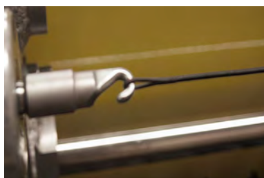
PSE's exclusive LiveWire™ bowstring machine stretches each individual strand to it's optimal tension.
