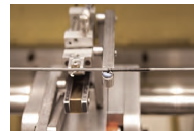
This automated process results in strings that have virtually zero stretch or peep rotation and are ultra-long lasting.
