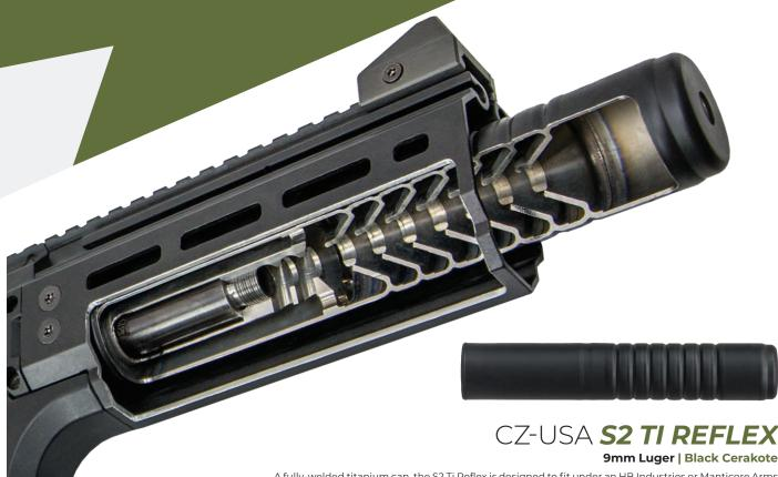
A fully-welded titanium can, the S2 Ti Reflex is designed to fit under an HB Industries or Manticore Arms handguard, allowing it to have a 2" reflex blast chamber and giving it the volume of much larger cans while only protruding from the muzzle 5.83 inches. This full titanium can weighs in at just 9.6 ounces and spits out 147-grain defensive loads at well under 130 dB
